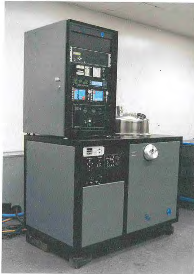
Example of a typical BJD-1800 Vacuum Deposition System
